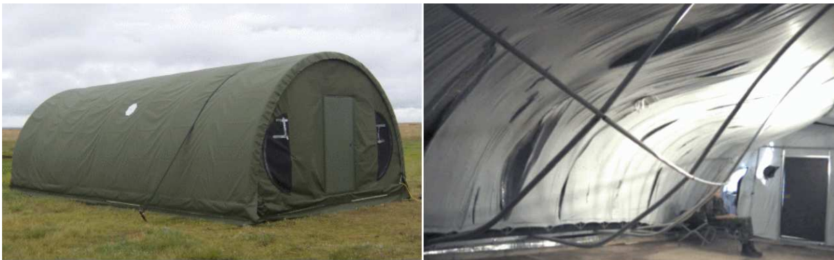
Typical hemi-cylindrical tent and internal snapshot of blast-response dynamics.
