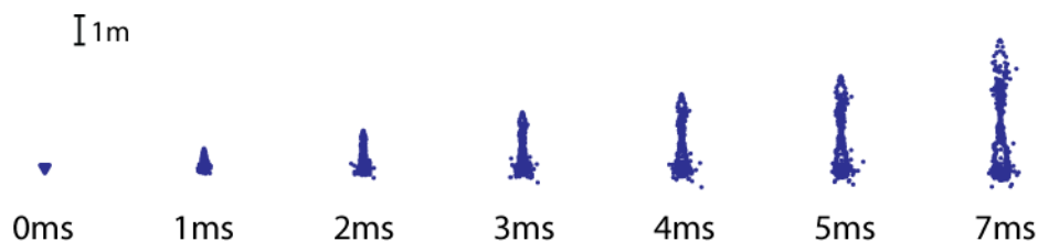
Fig. 2 Early time development of a jet of iron particles computed with the SPH method. Cone angle is 60° and m_{\text{iron}}/m_{\text{explosive}} = 14 .
