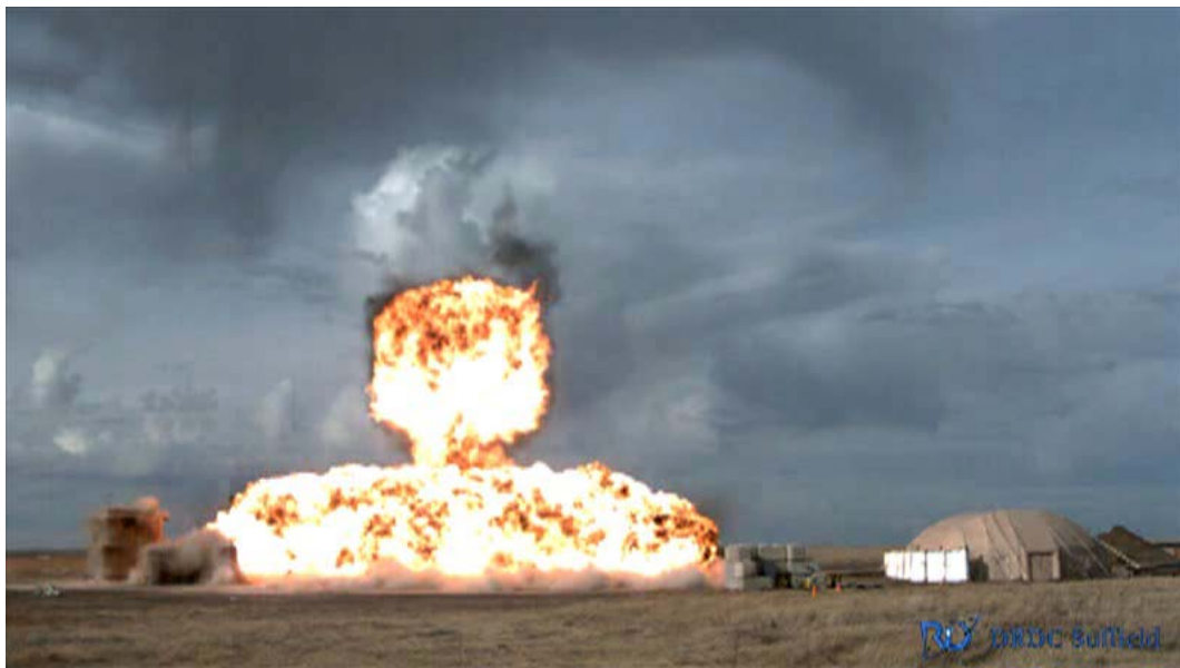
Blast field testing of the airbeam shelter system with integrated ballistic curainwall
