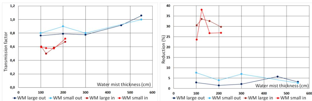
Figure 1. (Left) Transmission factor of initial overpressure and (Right) maximum impulse reduction versus the thickness of water mist which the blast wave passed in the both cases, detonation occurring inside (in) or outside the mist (out). Small: droplet diameter of 25-100  $\mu\text{m}$ . Large: droplet diameter of 200-300  $\mu\text{m}$ .
