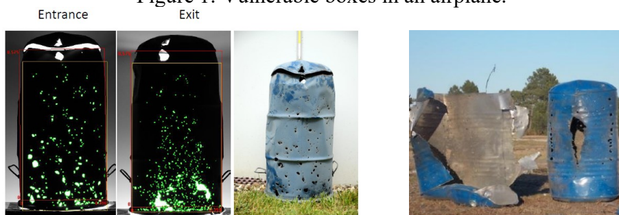
Figure 2: Evaluation procedure of perforated containers (left). Torn open containers on the front side (right).
