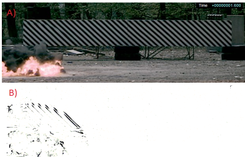
Figure 1: A) Frame from high-speed camera at 1.6 ms after trigger point B) Subtraction result of frames at 1.7 ms and 1.6 ms after trigger point
